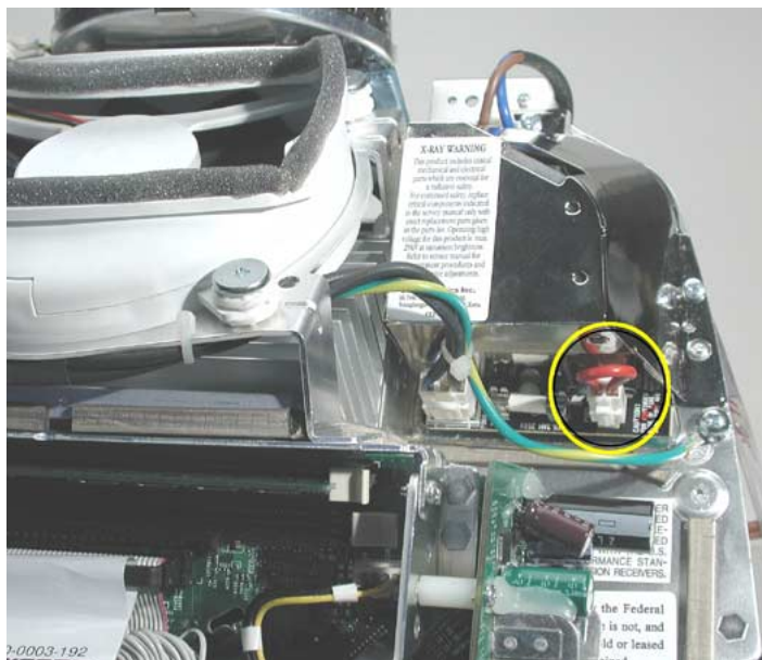
Figure 2: LHR Jumper Locator
