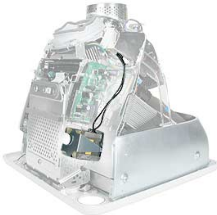
Figure 3: LHR Module Locator
